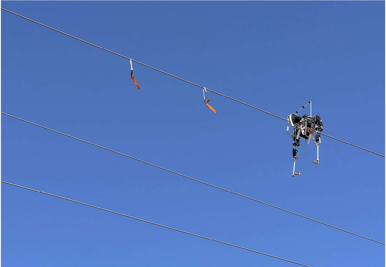
Figure 3 LiCAS dual arm rolling robot developed for the AERIAL-CORE project to perform the installation of bird flight diverters on power lines. The aerial transportation and retrieval of the arms is done using a multi-rotor through a hook-handle mechanism.
