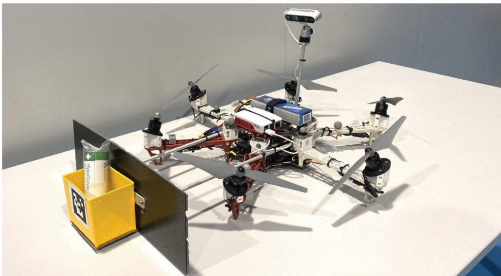
Figure 2 Prototype of fully-actuated aerial parcel delivery multi-rotor with front basket attached to the carbon fiber protection panel, and a Intel RealSense D435i camera for visual recognition of users.
