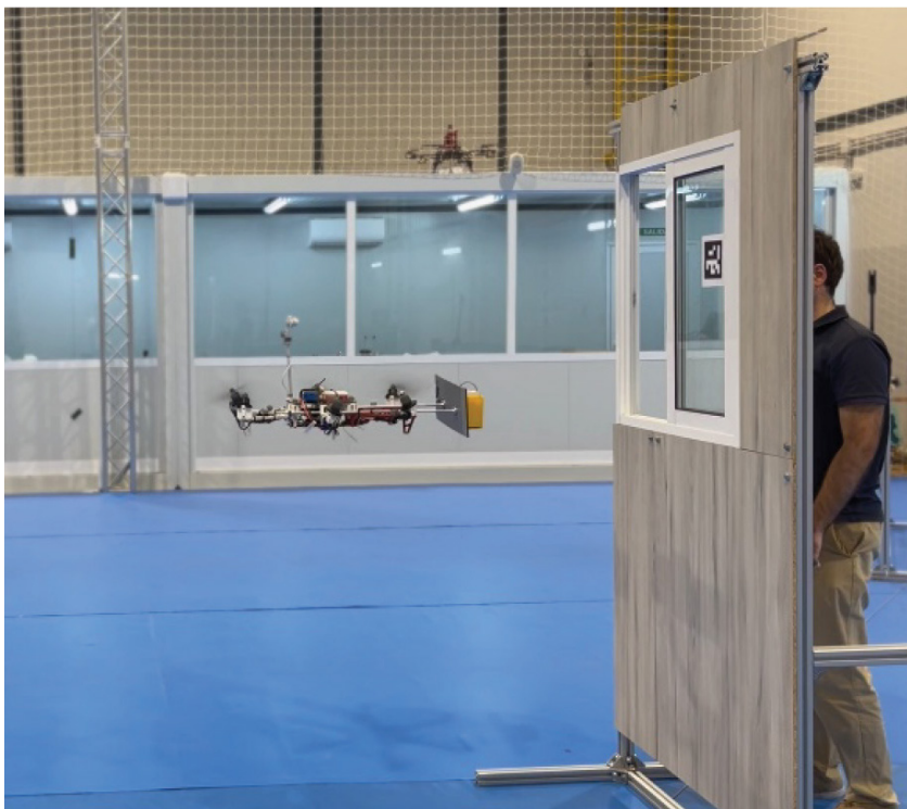
Figure 3 Evaluation scenario with the mock-up of a window within the GRVC Robotics Lab indoor testbed.
