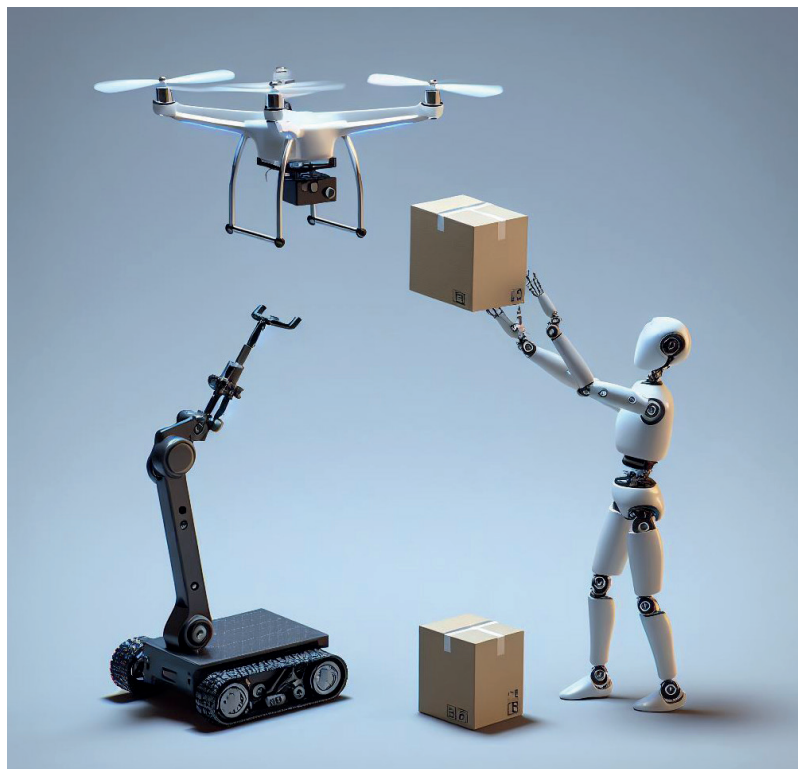
Figure 2: Handing a package from a drone to a humanoid robot or single-arm robot manipulator requires to reconcile drastically different perception, from different viewpoints and sensors, and distinct robot actions from unimanual to bimanual actions
